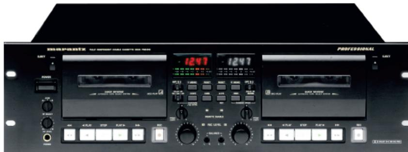
The Marantz Professional PMD510 is one of the most comprehensive and flexible dual well cassette decks specifically created for professional applications. Each of the two wells is a completely independent cassette deck (allowing simultaneous playback on well A while recording on well B or vice versa) with its own distinct set of stereo inputs and outputs, pitch control, stereo bargraph meters, a linear time counter, Dolby B/C selector, and large transport buttons.
